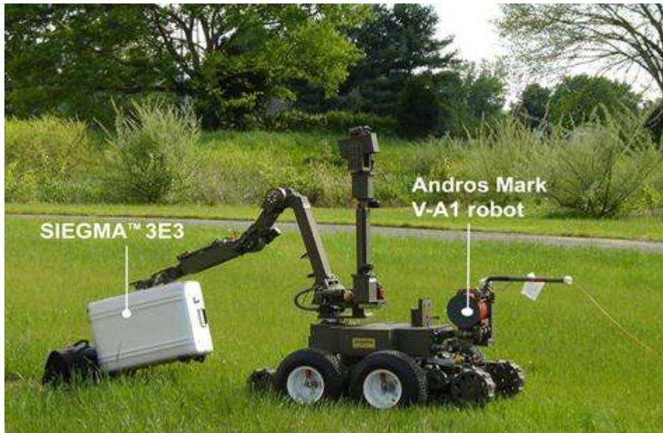
**FIGURE 4.** Robot-borne atometer “suitcase” model SIEGMA™ 3E3 inspects a briefcase, at Counter Terrorism in the Balkans Symposium, Belgrade, ( 2005). See open suitcase below.
