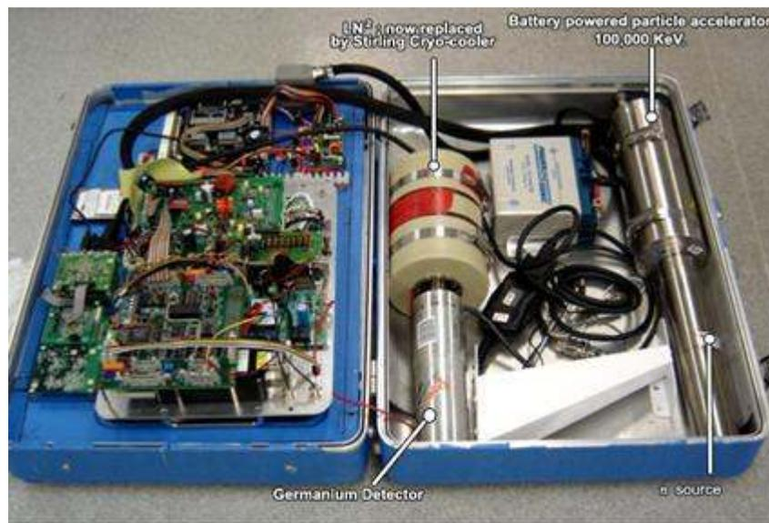
HiEnergy Technologies, Inc. Detector for Improvised Explosive Devices (IED): SIEGMA™.
